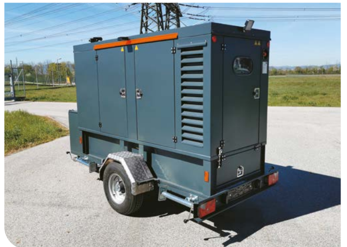
Mobile power generator
